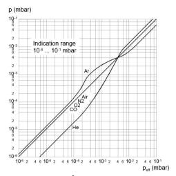
In the range below 10<sup>-5</sup> mbar, the pressure indication is linear. For gases other than air, the pressure can be determined by means of a simple conversion formula:
