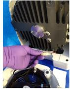
Remove 4 screws using 4 mm T-handle wrench to separate outboard housing from orbiting plate. Make sure pump is vented before attempting to separate scrolls.
