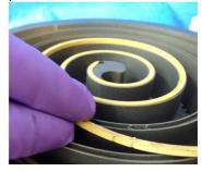
Apply a trace amount of grease (provided) on new O-ring and install.
