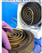
Clean both metal scrolls using abrasive scrubbing pad, low lint cloth, and low lint cleaning swabs. If a cleaning fluid is necessary or desired, use isopropyl alcohol (not included). Do not use water, detergent, or home/industrial cleaning products. Do not used compressed air or aero duster.
