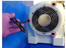
Remove front cowling and disconnect fan connector; set front cowling aside.
