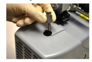
Remove 4 screws on front cowling using 4 mm T-handle wrench
