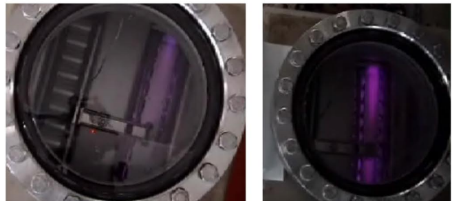
Figure 7. StarCell element. For voltages below approximately 1 kV, the discharge is contained within the ion pump element pocket.
