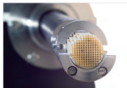
Intra-catalyst sampling of gas and temperature
