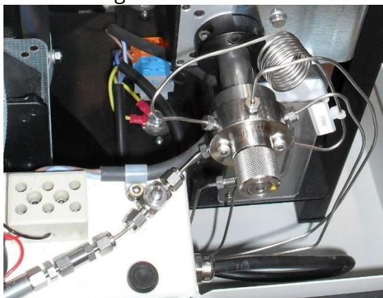
Figure 2 Capillary attached to outlet of valve
